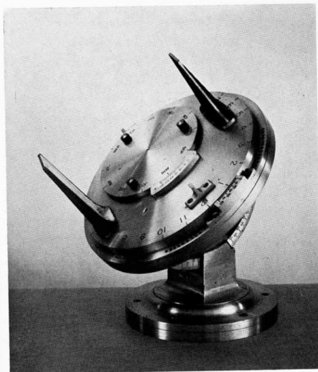
FIG. 100. Universal Helio-chronometer. Made and lent to the Science Museum (London), by Messrs. Pilkington & Gibbs, Ltd., Preston.
